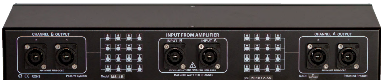
Speakon Inputs and Outputs with the guideline schematics for pin 2+/- for the Inputs and pin 1+ /1- for the Outputs. The manufacturer's intention was to eliminate the risk of confusion between Input and Output interfaces.
