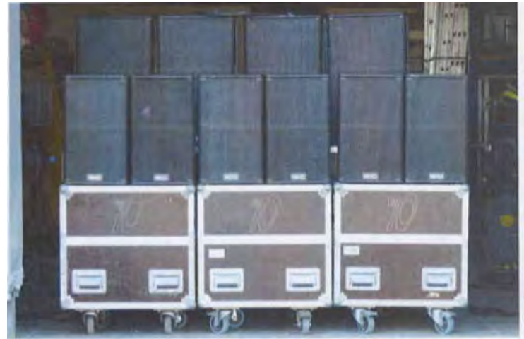
Outside of our testing room, the ten speakers used to load the Zero-Ohm unit on top of the two PS10s in front of the controls and amplifier
